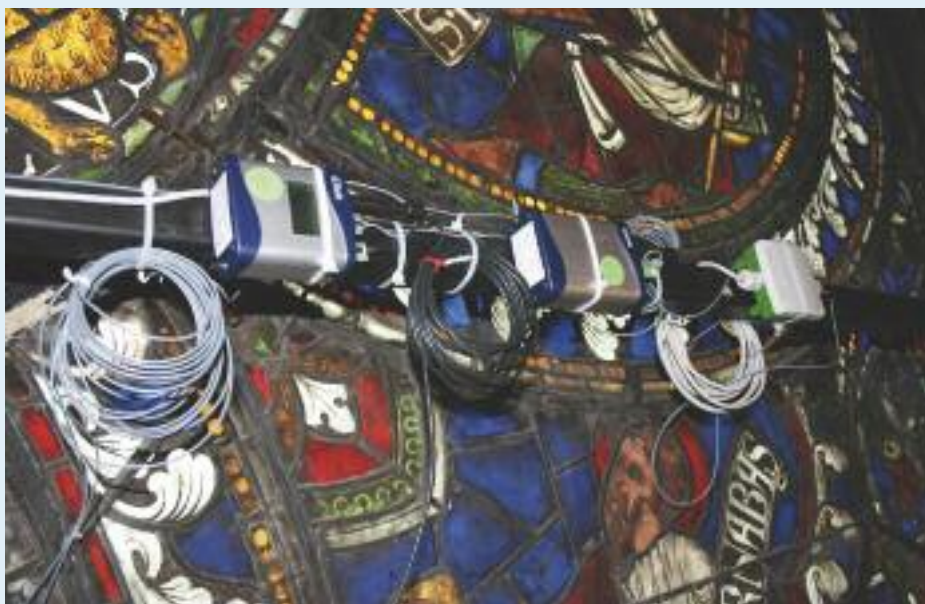
Transmitting equipment on Canterbury Cathedral's South Oculus window
