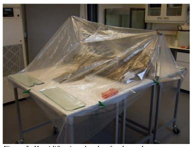
Figure 5: Humidification chamber for the parka
