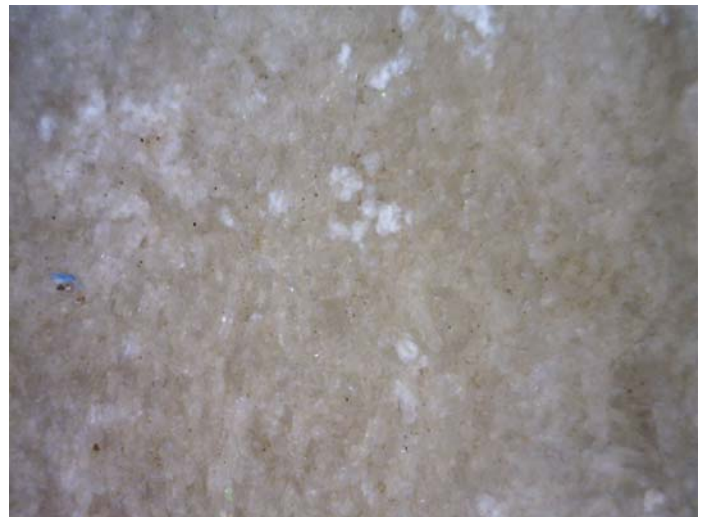
Detail of alabaster base of monument to William and Anne Clopton showing surface magnified x150 before and after cleaning
