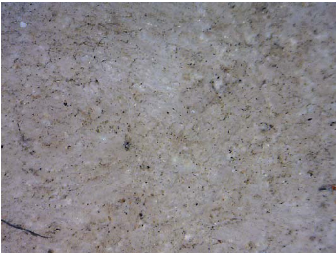
Detail of alabaster base of monument to William and Anne Clopton showing surface magnified x150 before and after cleaning
