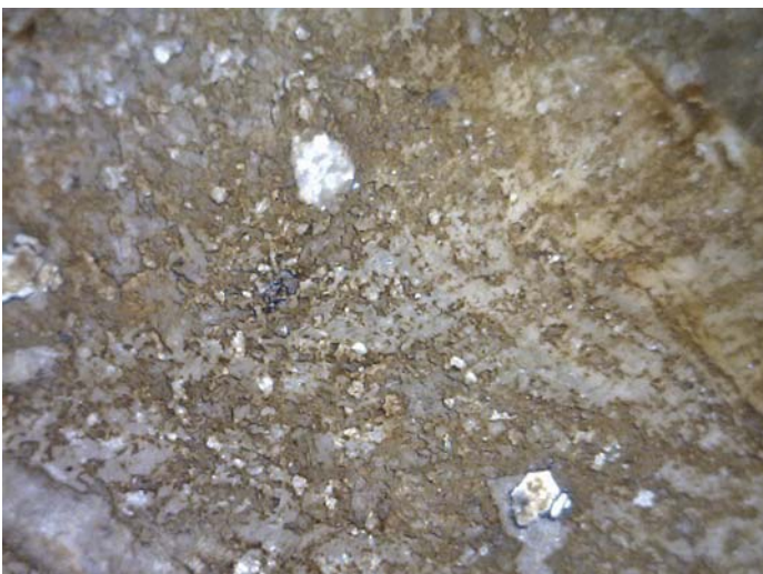
Detail of cushion of monument to William and Anne Clopton showing surface magnified x150 before and after cleaning; polychrome residues have been retained but the surface wax removed
