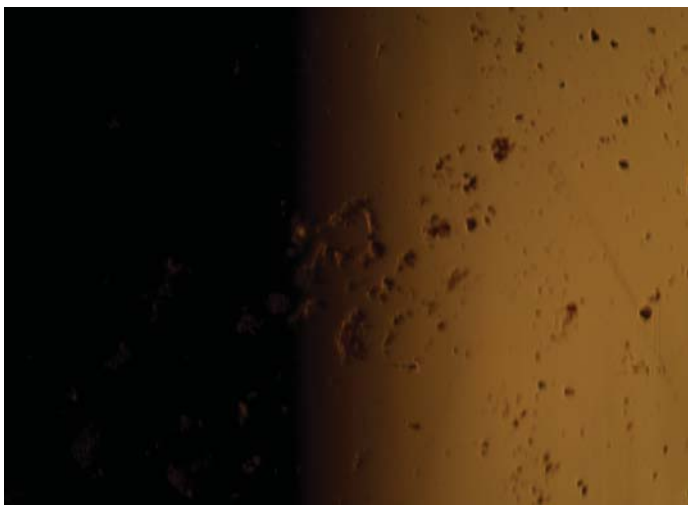
Figure 6 Yellow under modified Van der Kolk test
