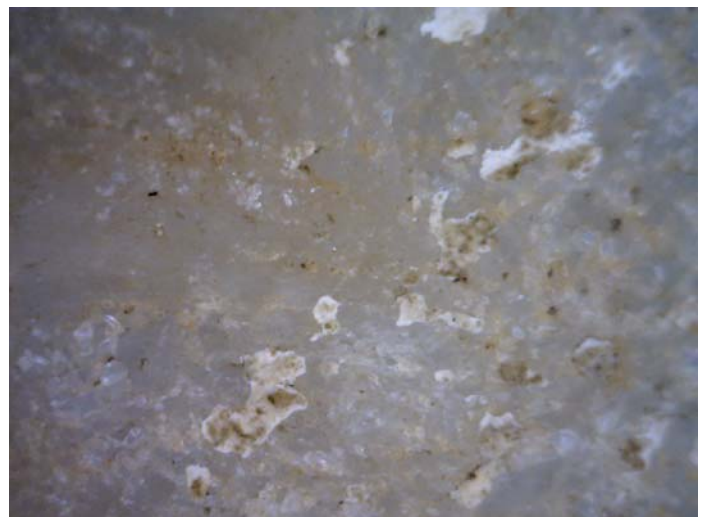
Detail of cushion of monument to William and Anne Clopton showing surface magnified x150 before and after cleaning; polychrome residues have been retained but the surface wax removed
