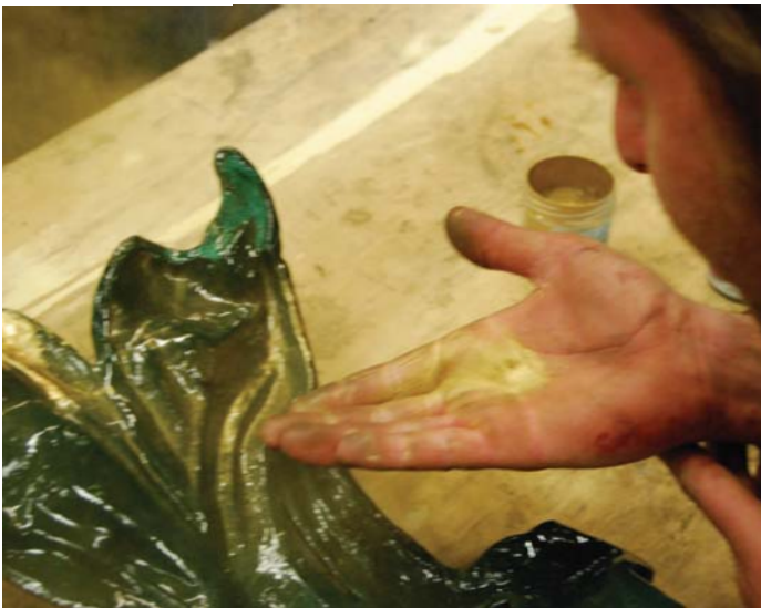
Blowing metallic powder over wet varnish
