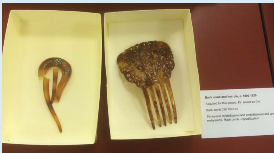
Plastic back comb and hair pin 1890–1920 suffering from crystallisation and other problems
